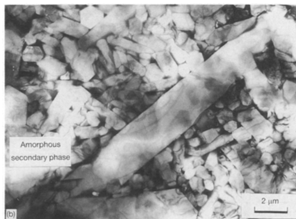
Figure 1 TEM micrographs of (a) sample Yb/A and (b) sample Y/S showing the general microstructures and grain morphologies. Note the much finer and globular shaped grains of sample Yb/A, shown in (a).
